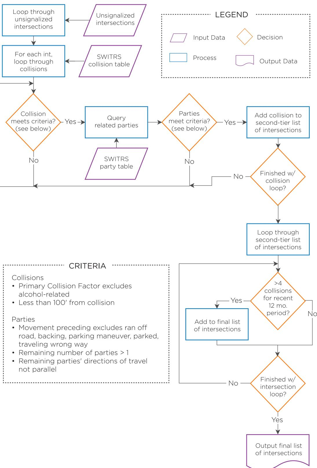
Example Process Diagram for Evaluation Tool (Step 3): This process diagram documents the method by which collisions are evaluated in the tool to determine if they qualify to be used in warranting signal improvements.
